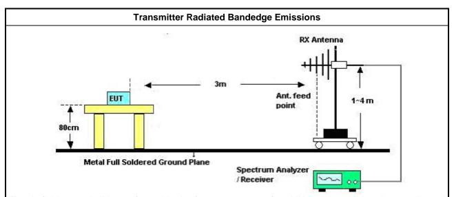
Electric field tests shall be performed in the frequency range of 30 MHz to 1000 MHz using a calibrated bi-log antenna. the antenna height shall be varied from 1 m to 4 m.
