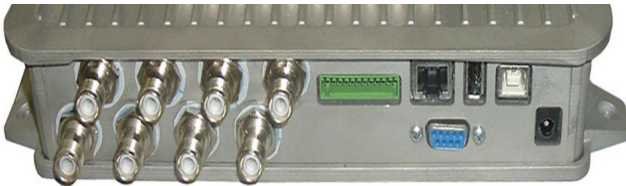
Figure 1-2 FX9500 Power and I/O Connections
