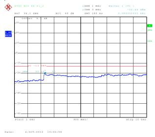
8.2.2.3 Out of Band Emissions at Antenna Terminals 1x EvDO BC1, Mid channel, 1880.0 MHz, 2 Hz to 1 GHz
