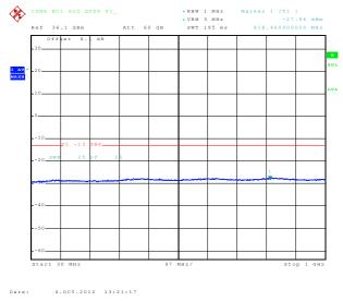
8.2.1.4 Out of Band Emissions at Antenna Terminals CDMA BC1, Mid channel, 1880.0 MHz, 1 GHz to 10 GHz
