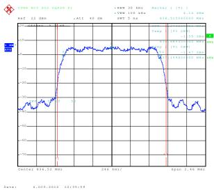
7.2.2.2 CDMA Occupied Bandwidth, SO2, RC3, BC0 Mid channel, 836.52 MHz, 99% BW
