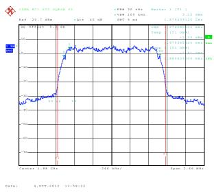
7.2.2.4 CDMA Occupied Bandwidth, SO2, RC3, BC1 Mid channel, 1880.0 MHz, 99% BW
