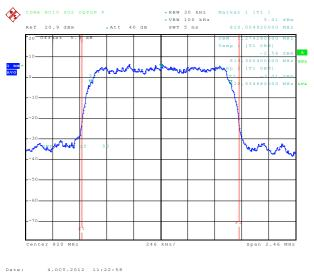
7.2.2.6 CDMA Occupied Bandwidth, SO2, RC3, BC10 Mid channel, 820.0 MHz, 99% BW
