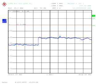
8.2.1.6 Out of Band Emissions at Antenna Terminals CDMA BC10, Mid channel, 820.0 MHz, 2 Hz to 1 GHz
