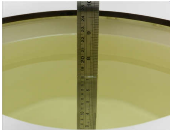
Fig 11.1 Photo of Liquid Height for Body SAR
