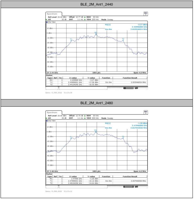
Note : The occupied channel bandwidth is maintained within the band of operation for all of the modulations.
