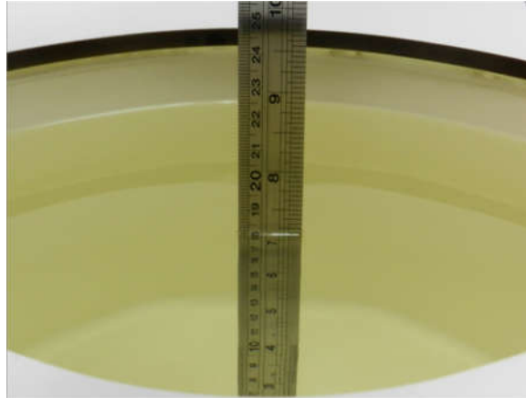
Fig 11.1 Photo of Liquid Height for Body SAR
