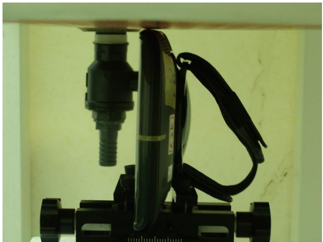
Primary Landscape with Phantom 0 cm Gap (EUT with Hand Strap)
