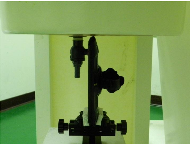
Primary Portrait with Phantom 0 cm Gap (EUT with Hand Strap and Jelly Sets)
