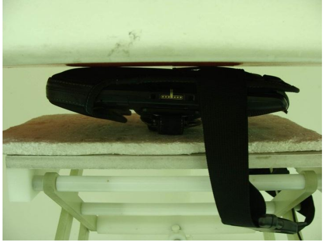
Front Face with Phantom 0 cm Gap (EUT with Holster and Hand Strap)
