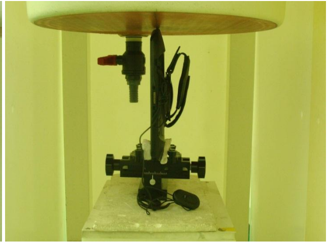
Secondary Portrait of DUT with phantom 0 cm gap (DUT with Hand strap)
