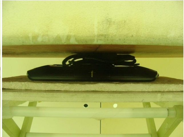
Bottom face of DUT with phantom 0 cm gap (DUT with Hand strap)
