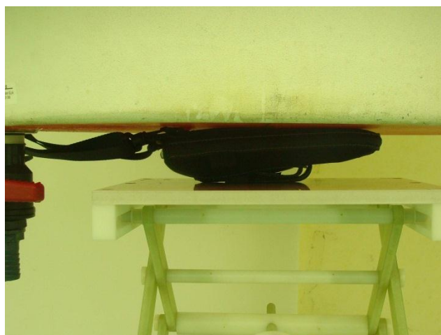
Front face of DUT with phantom 0 cm gap (DUT with Hand strap and Holster )
