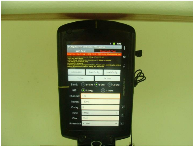
Secondary Portrait of DUT with phantom 0 cm gap
