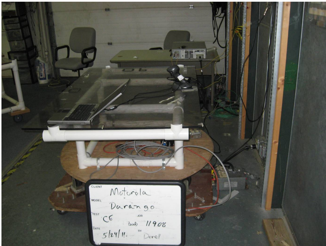
Photograph 4: Conducted Emissions Test Setup - Side
