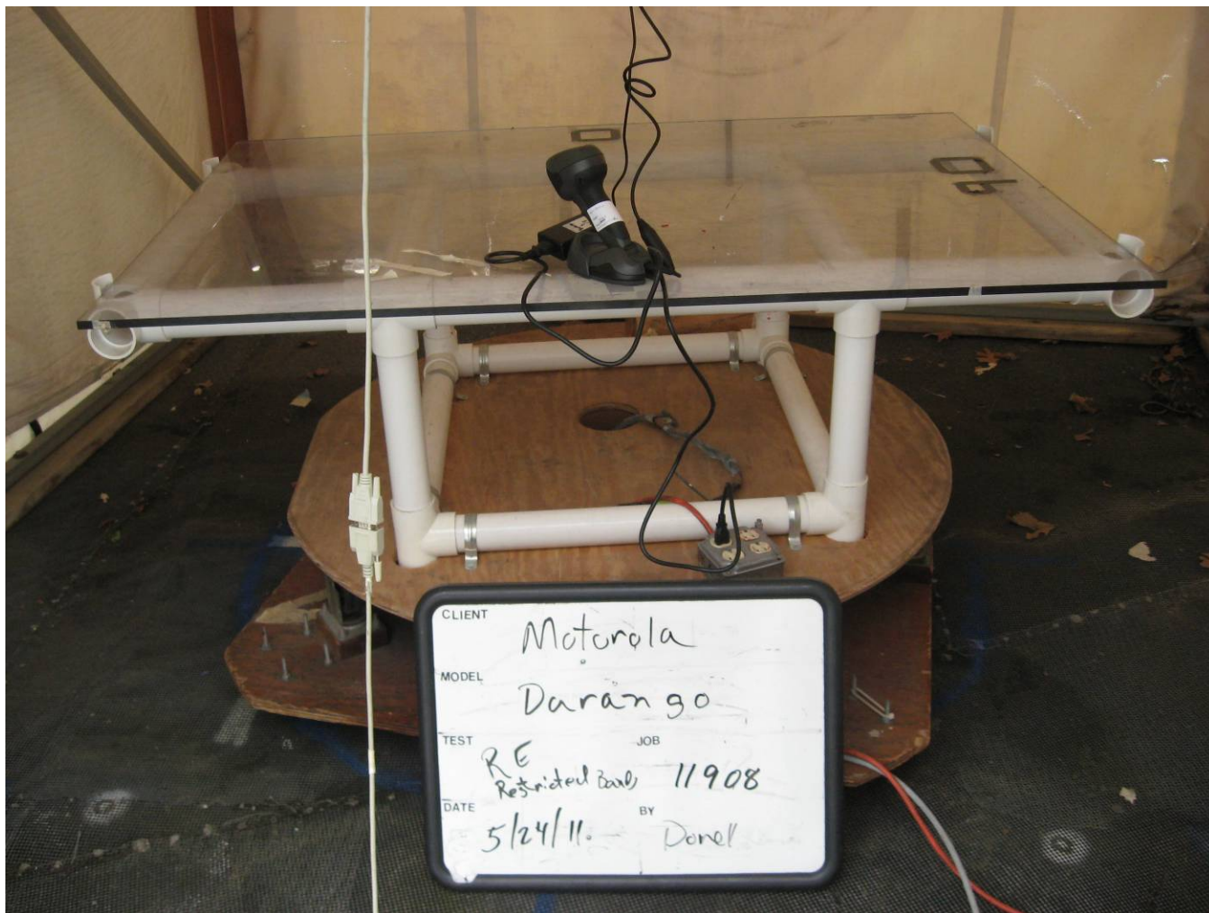
Photograph 2: Radiated Emissions Test Setup - Rear
