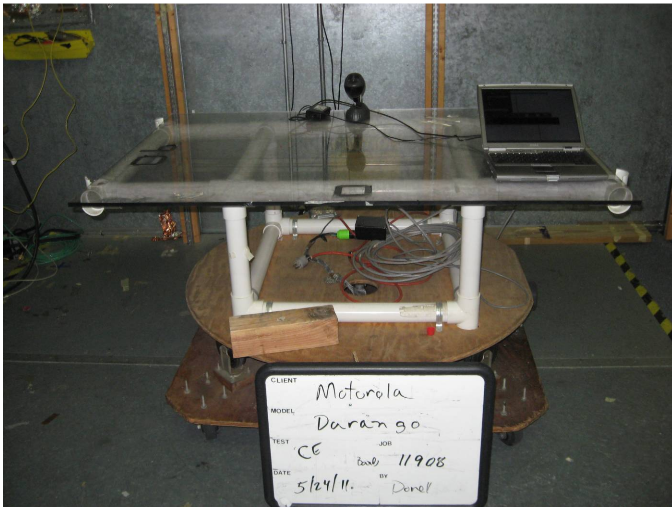
Photograph 3: Conducted Emissions Test Setup - Front
