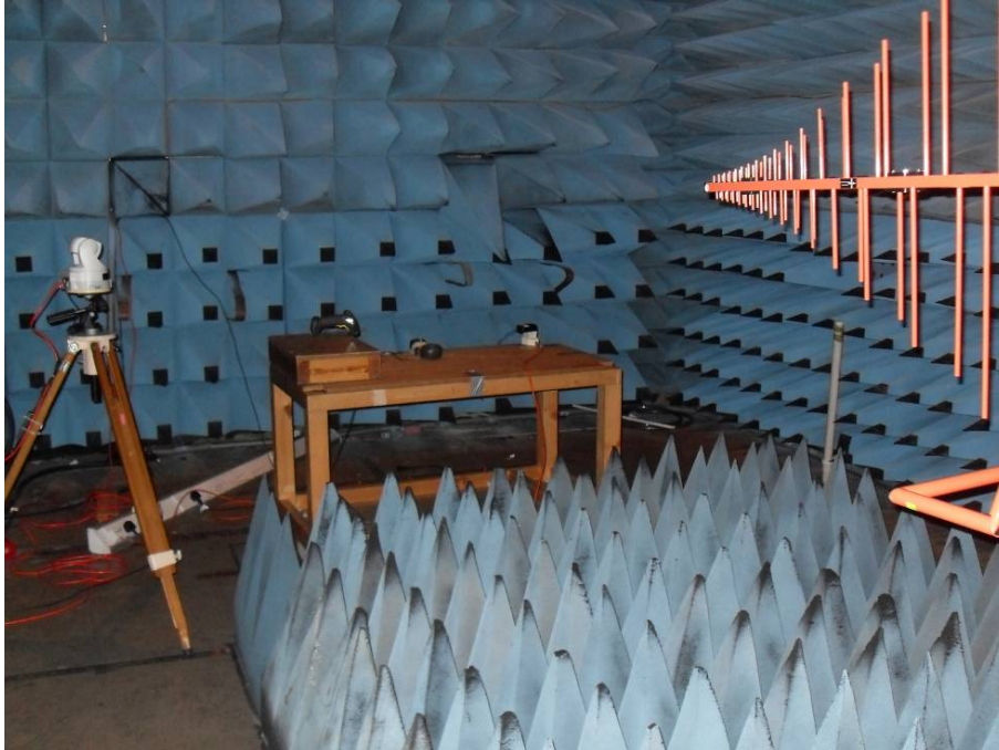
Immunity to Radio Frequency Electromagnetic Field (Enclosure Port)
