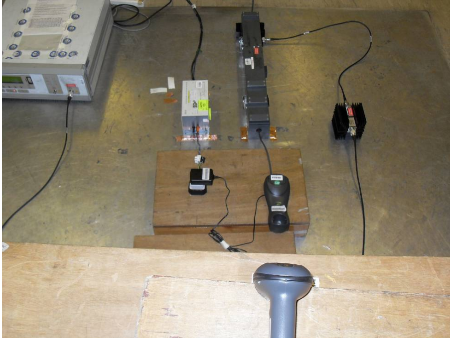
Immunity to Radio Frequency Common Mode (AC Power & Signal Ports)
