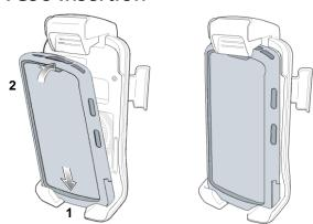
To ensure the TC58 is inserted correctly, align the device with the guard rails on the bottom of the cradle while inserting the device. Listen for the audible click that signifies that the TC58 locking mechanism is enabled and the TC58 is locked into place.
