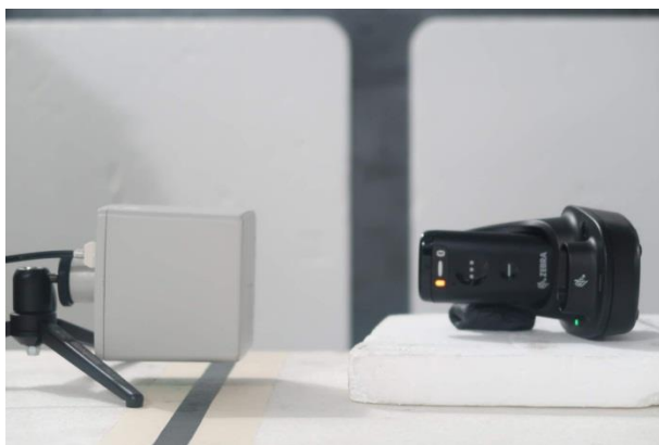
The Field Probe is placed 10cm distance to the front surface of EUT
