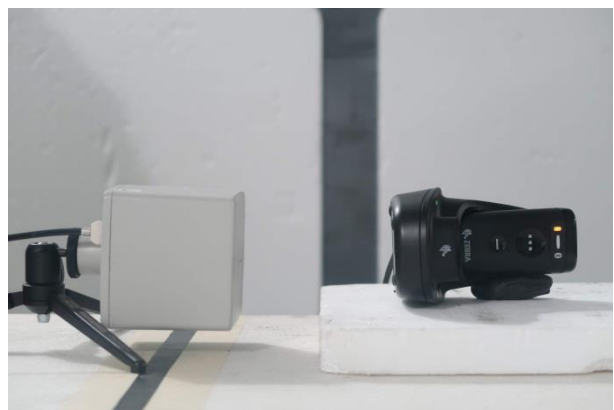
The Field Probe is placed 10cm distance to the front surface of EUT
