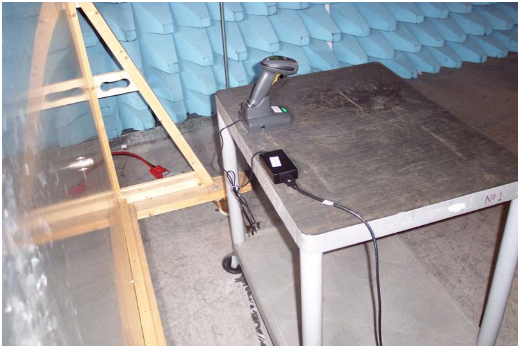
Config 1 – Stand Alone Conducted Emissions (AC Power Port)
