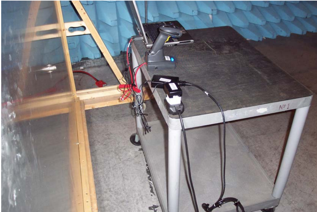
Config 2 – RS232 Conducted Emissions (AC Power Port)
