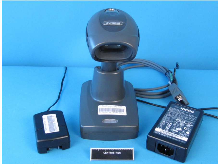
EUT (Cradle shown here with its (HIPRO) PSU, Scanner and RS232 Cable & PSU)
