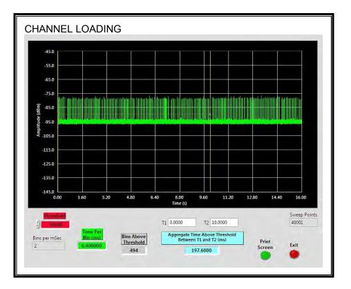
The level of traffic loading on the channel by the EUT is 1.976%
