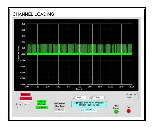
The level of traffic loading on the channel by the EUT is 1.76%
