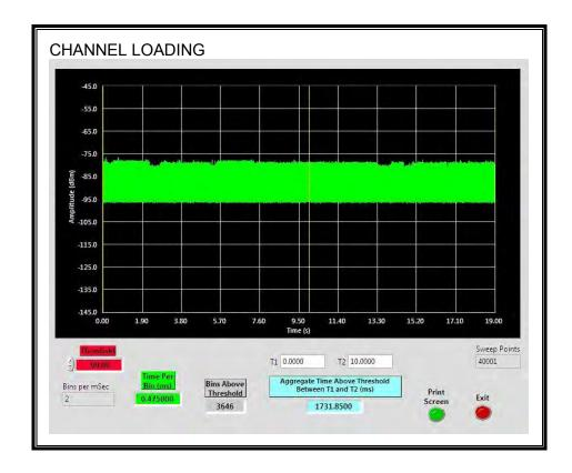
The level of traffic loading on the channel by the EUT is 17.3185%
