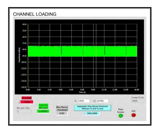
The level of traffic loading on the channel by the EUT is 18.82%
