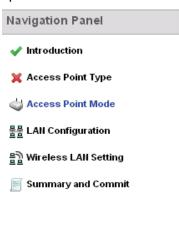
A green checkmark to the left of an item in the **Navigation Panel** defines the task as having its minimum required configuration set correctly. A red X defines a task as still requiring at least one parameter be defined correctly.
