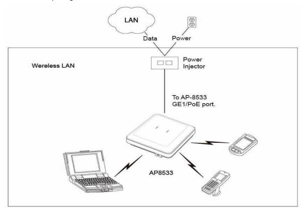
The Power Injector can be installed free standing, on an even horizontal surface or wall mounted using the Power Injector's wall mounting key holes. The following guidelines should be adhered to before cabling the Power Injector to an Ethernet source and an Access Point:
