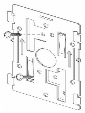
4. Place the Access Point on the mounting bracket.
