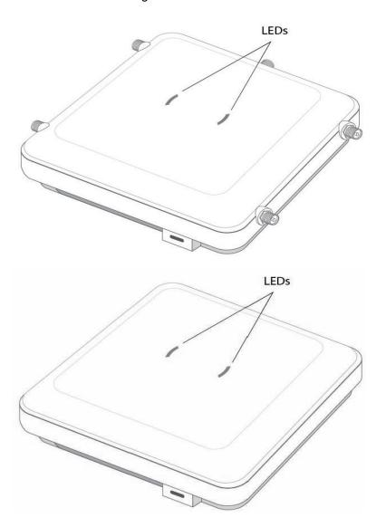
The LEDs display error conditions, and transmission, and network activity for the 5 GHz 802.11ac (amber) radio and the 2.4 GHz 802.11n (green) radio.
