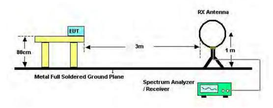
For Radiated Emissions: 30MHz~1GHz
