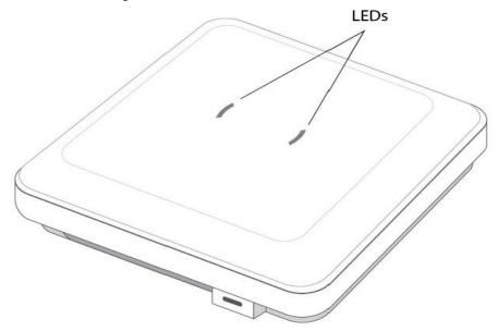
The LEDs display error conditions, and transmission, and network activity for the 5 GHz 802.11ac (amber) radio and the 2.4 GHz 802.11n (green) radio, sensor radio (white) and the BLE radio (blue).
