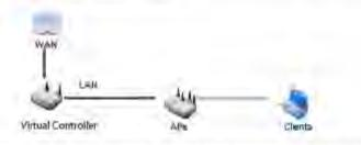
Bridge Mode - In Bridge Mode, the access point depends on an external router for routingLAN and WAN traffic. Routing is generally used on one device, whereas bridging is typically used in a larger density network. Thus, select Bridge Mode when deploying this access point with numerous peer APs supporting clients on both the 2.4 and 5GHz radio bands.
