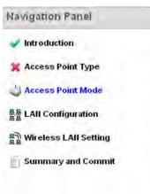
A green checkmark to the left of an item in the **Navigation Panel** defines the task as having its minimum required configuration set correctly. A red X defines a task as still requiring at least one parameter be defined correctly.
