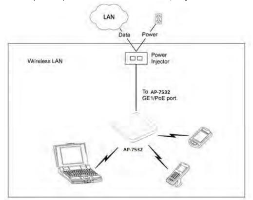
The Power Injector can be installed free standing, on an even horizontal surface or wall mounted using the power injector's wall mounting key holes. The following guidelines should be adhered to before cabling the Power Injector to an Ethernet source and an Access Point:
