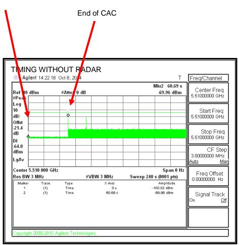
Transmissions begin on channel after completion of the CAC period.
