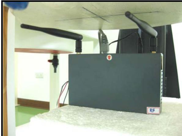
The edge of the EUT face to the phantom with 10mm-separation distance.
