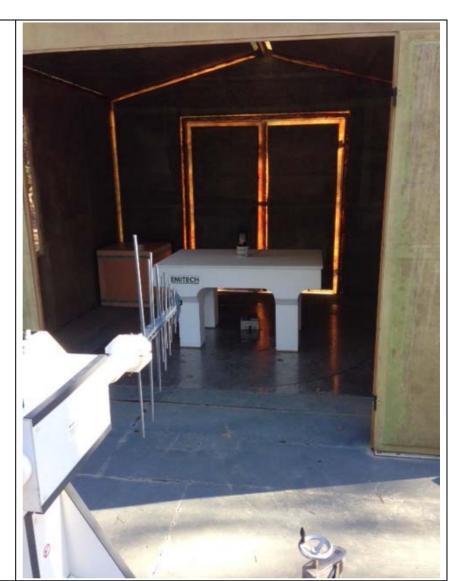
Radiated measurement on open area test site
