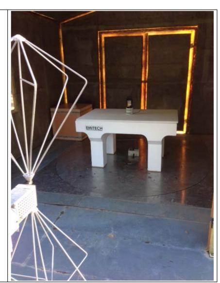
Radiated measurement on open area test site
