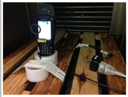
Ac power supply used for 110Vac/60Hz power supply measurement
