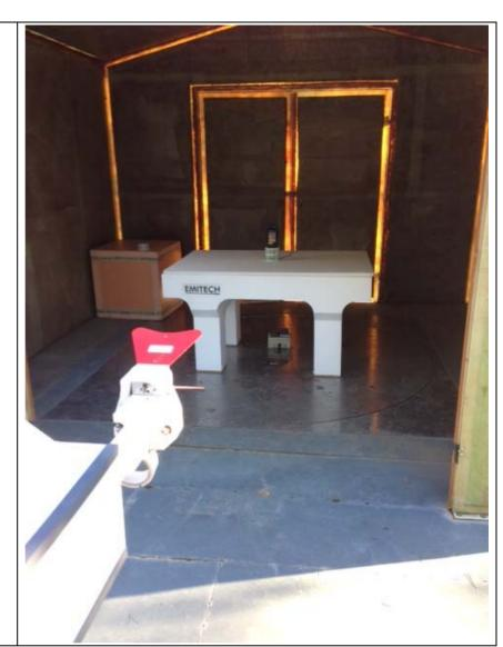
Radiated measurement on open area test site
