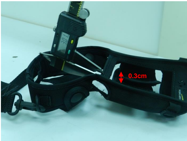
Carry Case(Model Name: WA6080)_ RF exposure configuration Front 0.3cm
