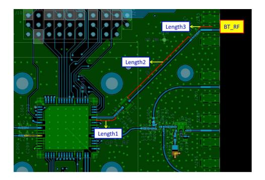
Different antenna length and shapes affect radiated emissions and each design shall be considered a different type; e.g., antenna length in multiple(s) of frequency wavelength and antenna shape (traces in phase) can affect antenna gain and must be considered;
