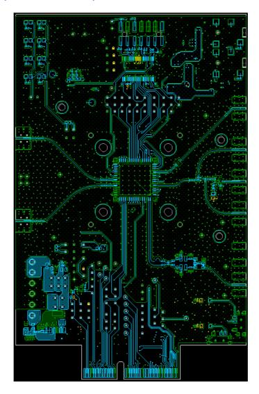
The critical transmitted microstrip lines are the RF2, RF1, BT\_RF.
