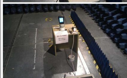
Radiated electric emission (pre measurement)
