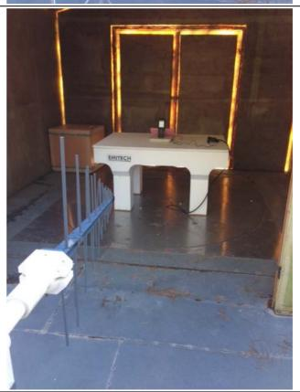
Radiated measurement on open area test site
