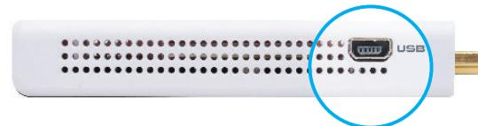
If the source does not have a USB port that can provide power to the Sender unit, connect the 5V/1A power supply.
