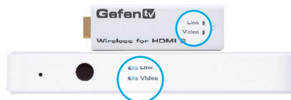
6. If the Sender and Receiver units do not pair automatically, point the IR remote at the IR sensor window on the Receiver and press Menu. Navigate through the on-screen menu and have the Receiver look for a Sender. Press and hold the pairing button on the Sender until the Link LED stops blinking. Press OK on the remote. A message indicating that the Sender and the Receiver have been paired will appear on the display.
