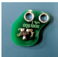
Figure 6: Hall Sensor Board, Front
