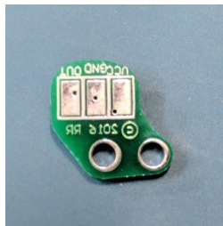
Figure 5: Hall Sensor Board, Back
