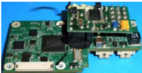
Figure 6: Main Board stacked with COTS Command Receiver
