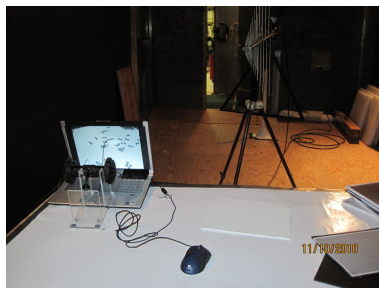
(a) Full test apparatus with testing antenna shown.
