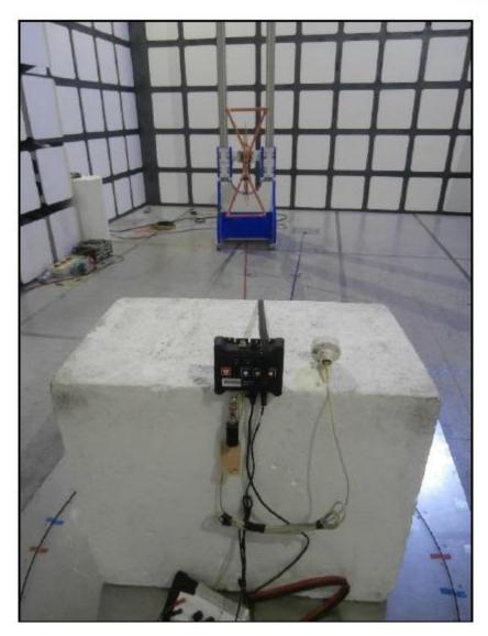
Figure 3: 30 MHz to 1GHz, EUT Orientation Y
