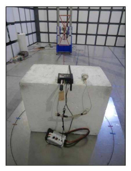
Figure 1 – 30 MHz to 1 GHz, EUT Orientation X
