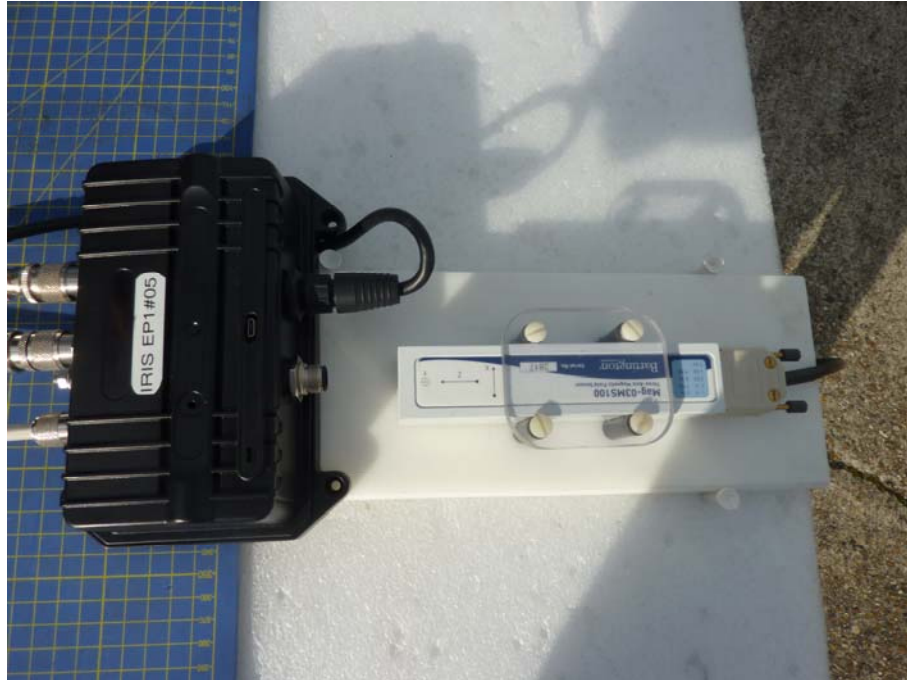
Compass Safe Distance Test Set-ups
