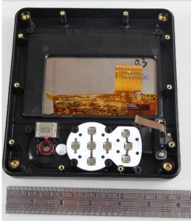
Figure 13 – Front Panel Internal view
