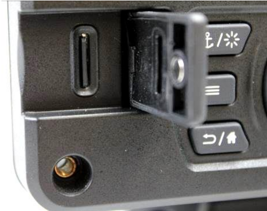
Figure 5 – SD Card location
