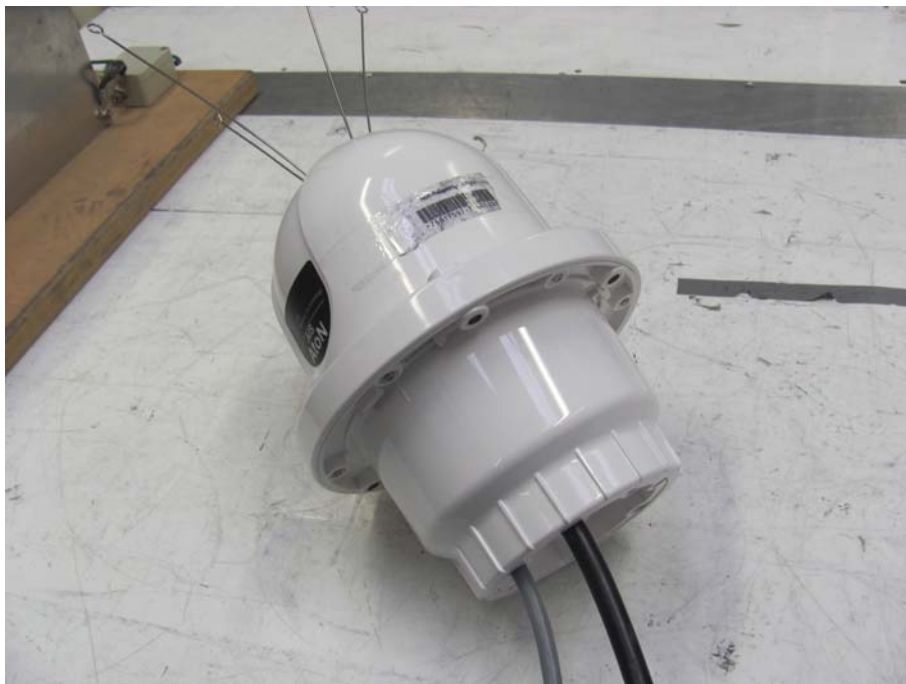
Immunity to Electrostatic Discharge (Enclosure Port)
