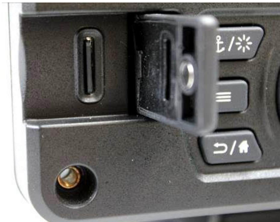
Figure 5 – SD Card location
