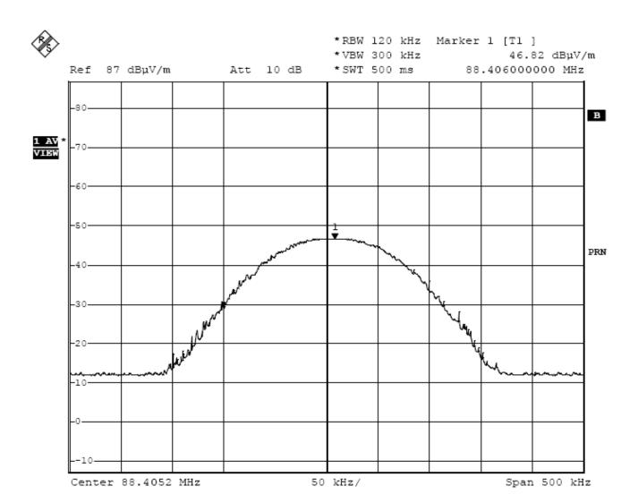
Comment B: Manuf:Kingsun EUT:Wireless Headphone M/N:MF-210 Memo :TX Antenna Polarization:Vertical
