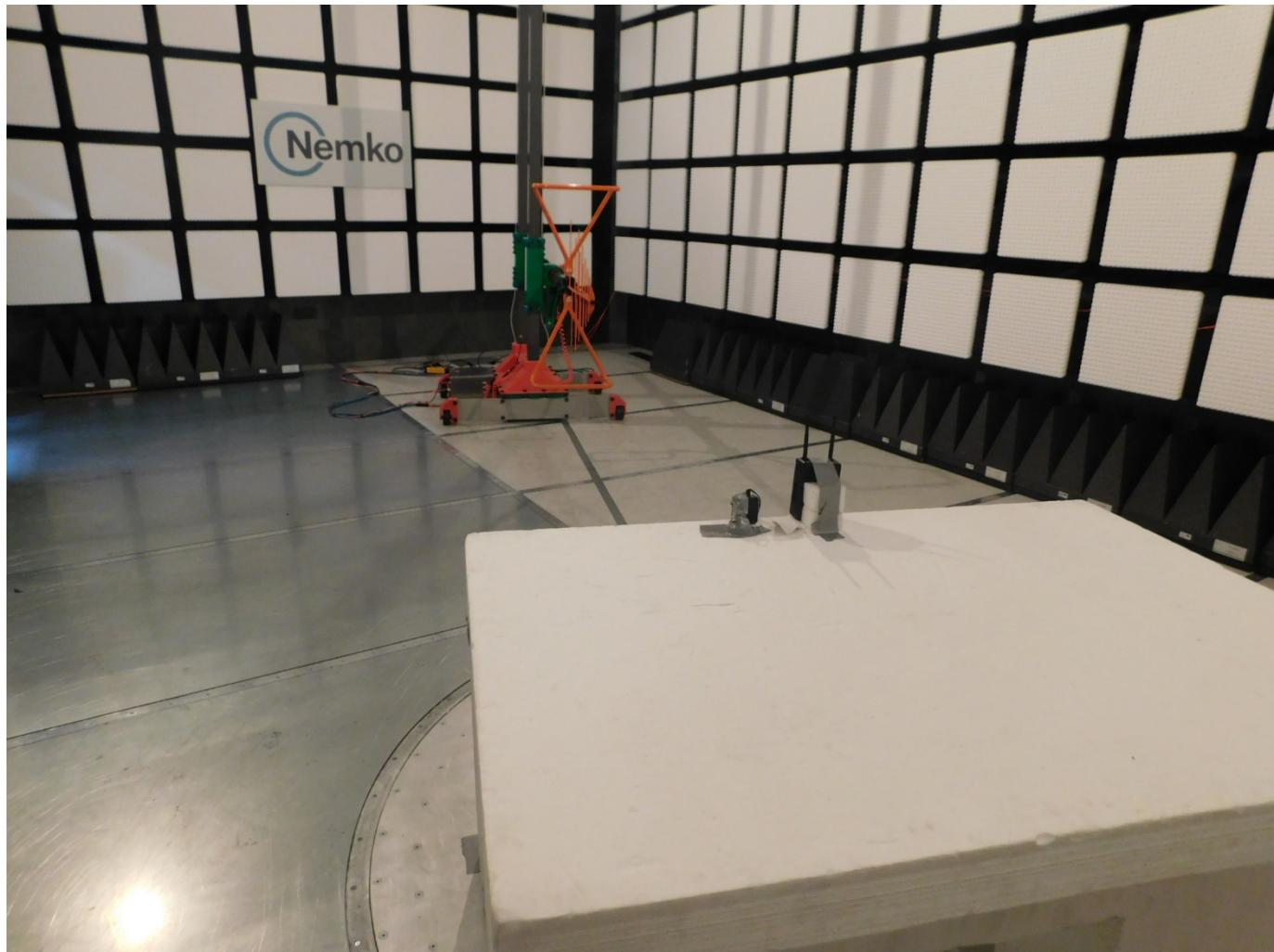
1.3 Radiated emissions above 1 GHz, Front view
