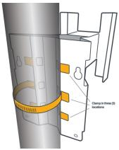
3. Attach the W4005 adapter with the attached mounting plate to the mounting hardware.
