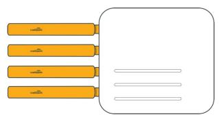
**NOTE**: Do not connect any antennas to the RP-SMA WiFi connections. If antennas must be connected, use only Cradlepoint 170628-000 2.7dBi dipole antenna, or another dipole antenna with lower gain.
