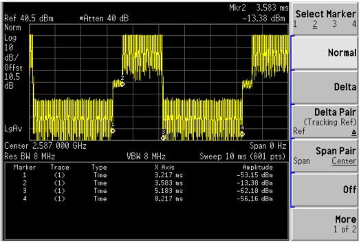
Burst lengh = Mark4 - Mark1=8.217ms- 3.217ms = 5ms 15 symbols UL = Mark3 - Mark2 = 5.183ms-3.583ms = 1.6ms Duty cycle = 1.6 / 5 \*100 % = 32 %
