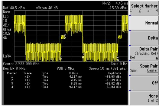
Burst lengh = Mark4 – Mark1=9.117ms- 4.117ms = 5ms 15 symbols UL = Mark3 – Mark2 = 6.05ms-4.45ms = 1.6ms Duty cycle = 1.6 / 5 \*100 % = 32 %
