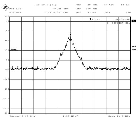
Figure 16 - Band-edge Measurement, High Channel, Fundamental
