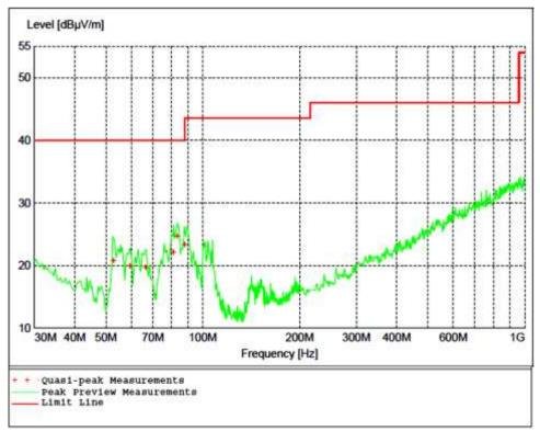
Figure 5 - Radiated Emissions Plot, High Channel Vertical orientation was found to be the worse-case
