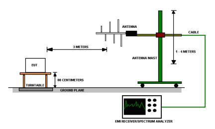
Figure 1 - Radiated Emissions Test Setup
