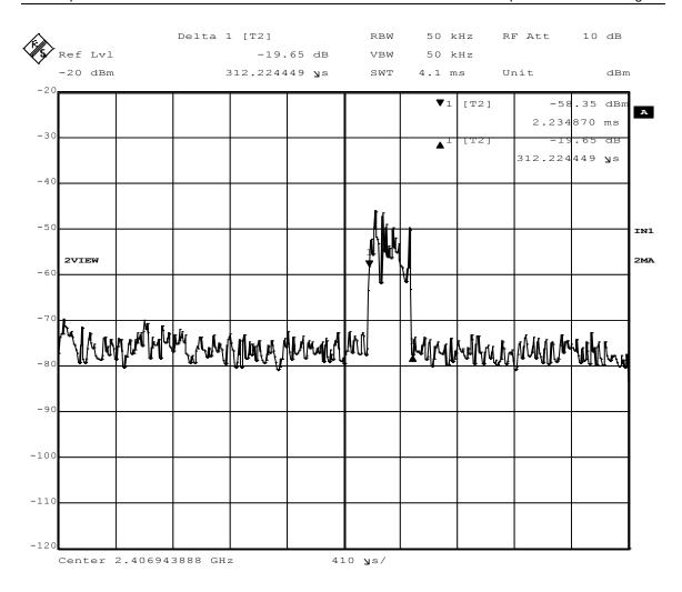
Figure 8 - Maximum Pulse Width
