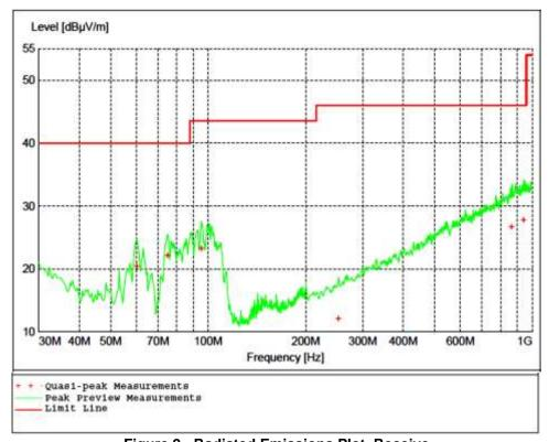
Figure 2 - Radiated Emissions Plot, Receive
