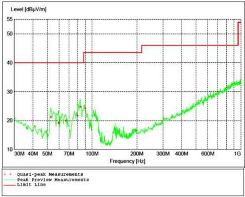
Figure 4 - Radiated Emissions Plot, Mid Channel Vertical orientation was found to be the worse-case
