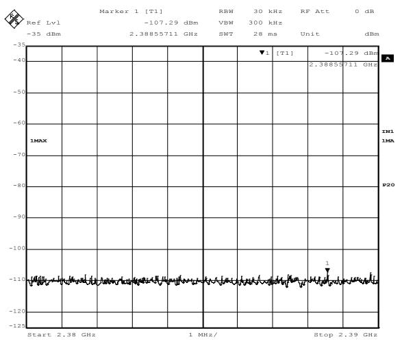
Figure 13 - Band-edge Measurement, Low Channel, Restricted Frequency
