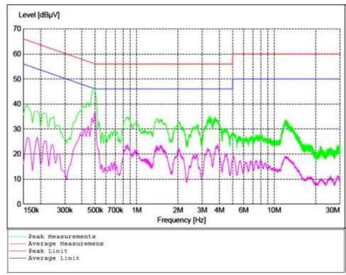
Figure 18 - Conducted Emissions Plot
