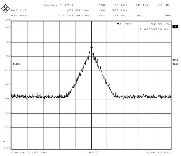
Figure 14 - Band-edge Measurement, Low Channel, Fundamental
