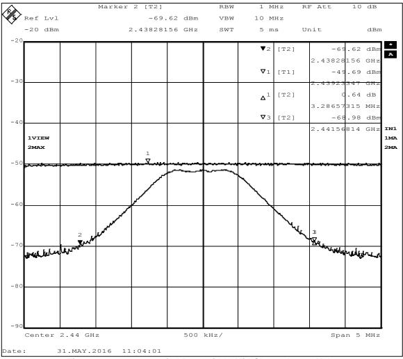
Figure 11 - 99% Occupied Bandwidth, Mid Channel, 3.28 MHz
