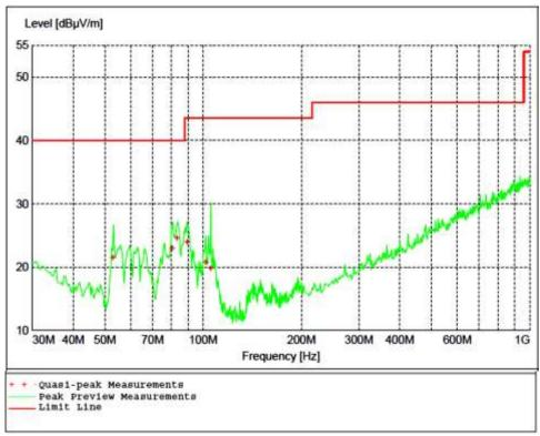
Figure 3 - Radiated Emissions Plot, Low Channel Vertical orientation was found to be the worse-case
