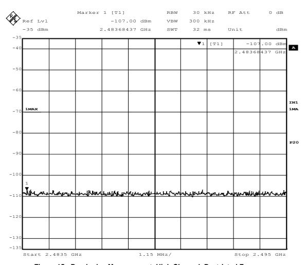
Figure 15 - Band-edge Measurement, High Channel, Restricted Frequency
