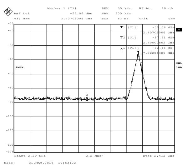
Figure 17 - Band-edge Measurement, High Channel, out-of-band
