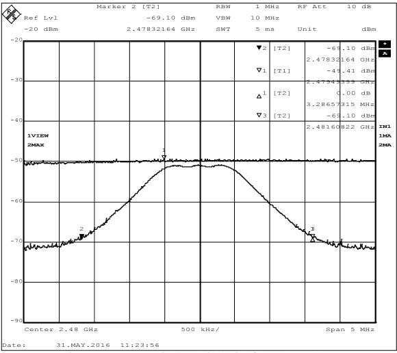
Figure 12 - 99% Occupied Bandwidth, High Channel, 3.28 MHz
