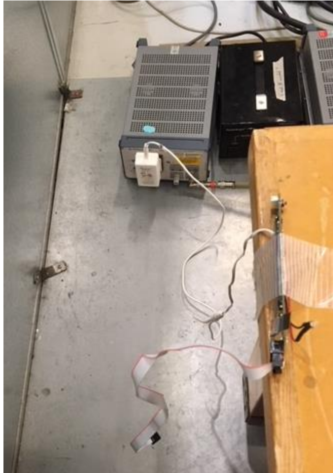
Figure 7 – Conducted Emissions Test Setup
