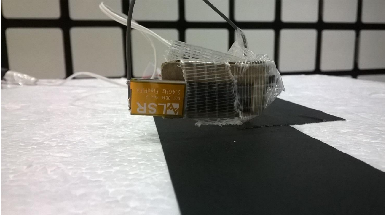
Figure 4 - Radiated Emissions Test Setup, Y axis
