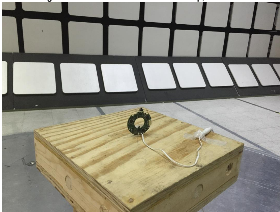
Figure 18 - Radiated Emissions Test Setup, Vertical
