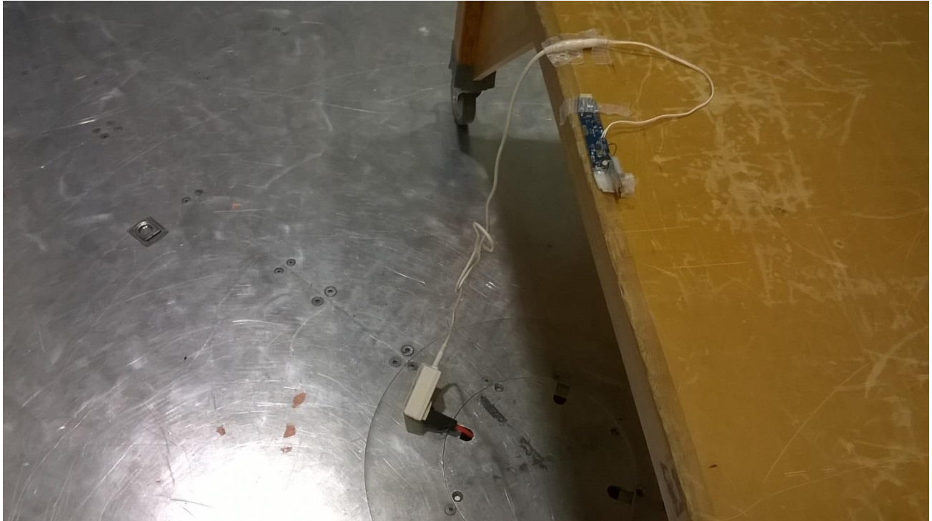
Figure 1 - Radiated Emissions Test Setup, 30MHz - 1GHz
