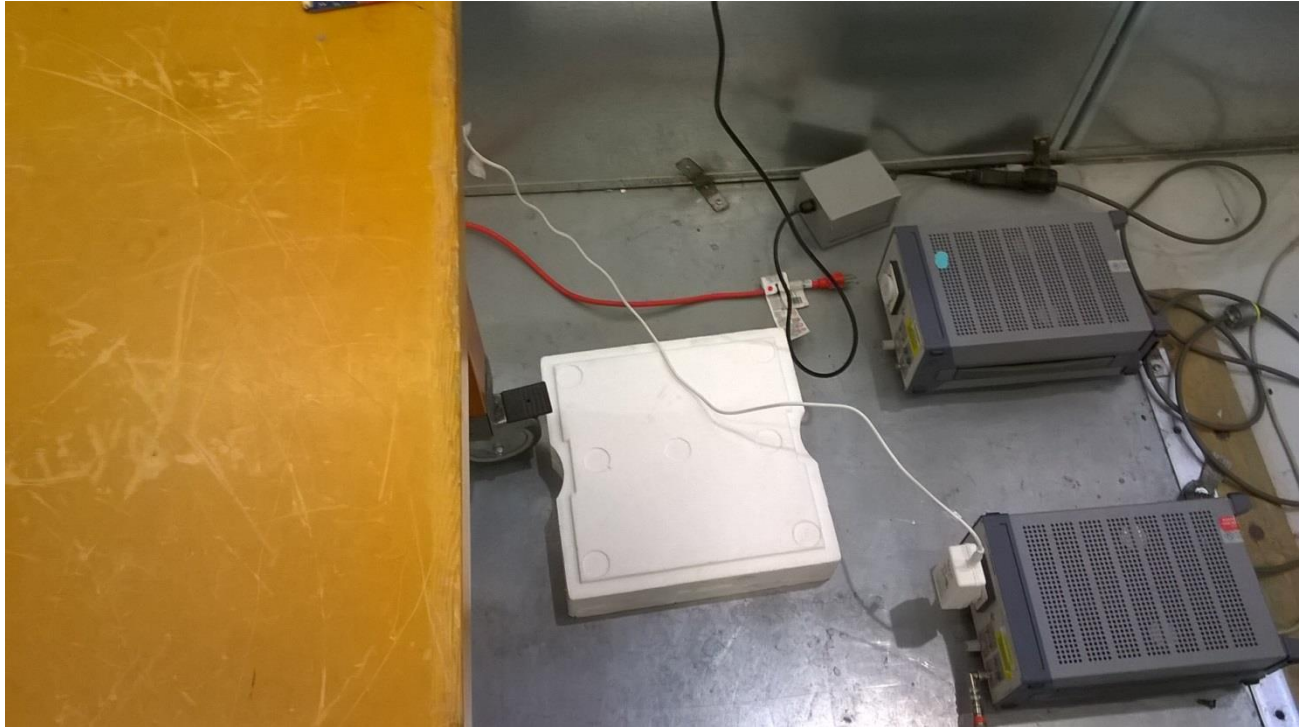
Figure 8 – Conducted Emissions Test Setup
