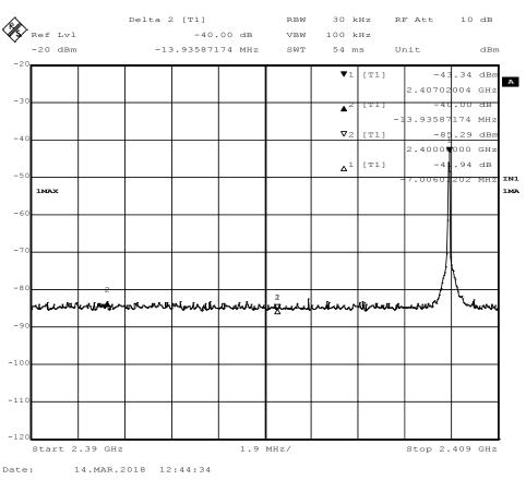
Figure 21 - Band-edge Measurement, Low Channel, Fundamental, Radiated Measurement The plot shows an uncorrected measurement, used for relative measurements only.
