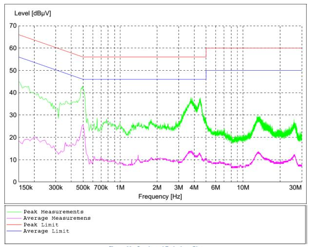
Figure 28 - Conducted Emissions Plot All measurements were found to be at least 10dB below the applicable limit.
