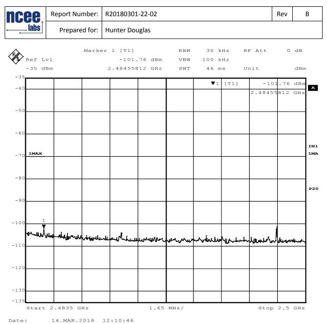
Figure 23 - Band-edge Measurement, High Channel, Restricted Frequency, Radiated Measurement The plot shows an uncorrected measurement, used for relative measurements only.
