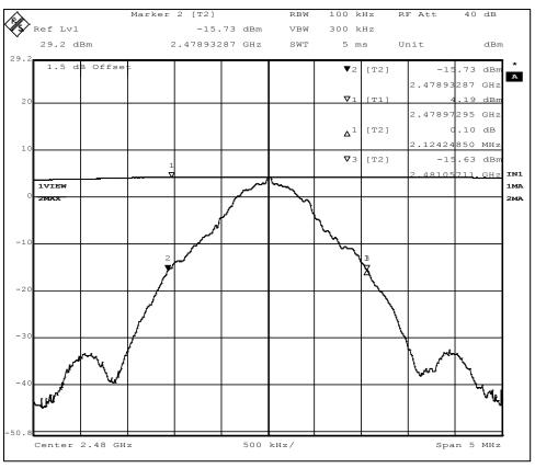
Figure 16 - 99% Occupied Bandwidth, High Channel
