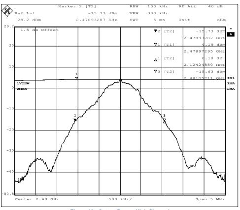
Figure 12 - Output Power, High Channel
