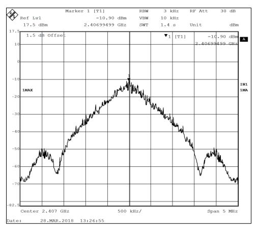
Figure 25 - Power Spectral Density, Low Channel
