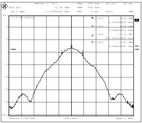
Figure 19 - 6dB Bandwidth, High Channel
