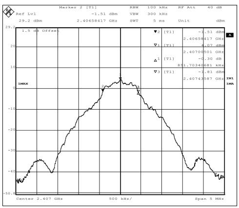
Figure 17 - 6dB Bandwidth, Low Channel
