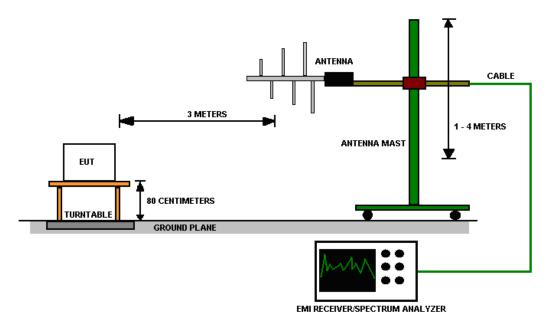
Figure 4 - Radiated Emissions Test Setup
