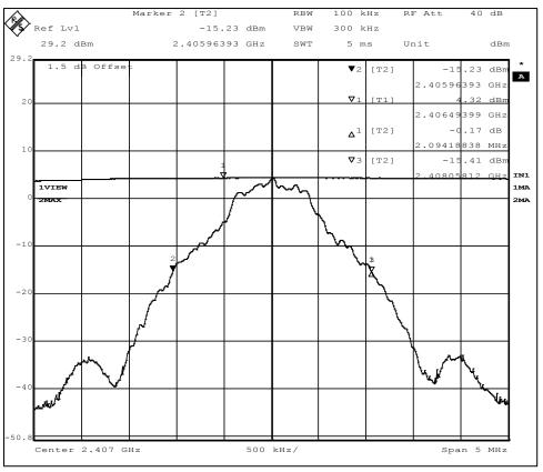
Figure 14 - 99% Occupied Bandwidth, Low Channel
