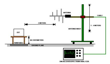
Figure 1 - Radiated Emissions Test Setup
