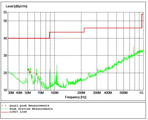
Figure 7 - Radiated Emissions Plot, Mid Channel
