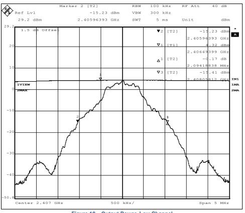
Figure 10 – Output Power, Low Channel
