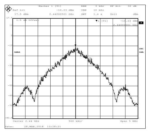
Figure 26 - Power Spectral Density, Mid Channel
