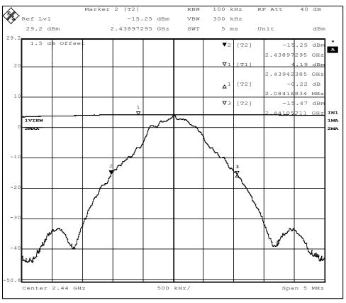
Figure 15 - 99% Occupied Bandwidth, Mid Channel
