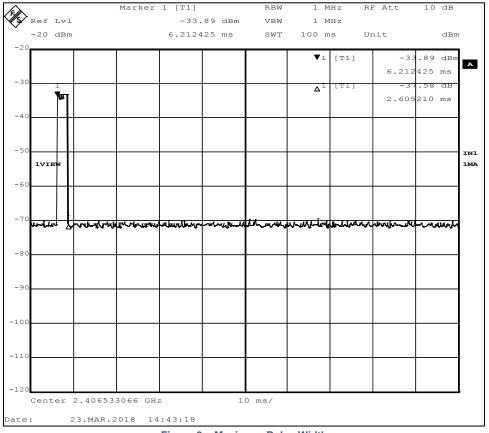
Figure 3 – Maximum Pulse Width
