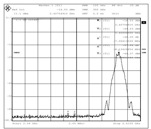
Figure 22 - Band-edge Measurement, Low Channel, Unrestricted Frequency, Conducted Measurement The plot shows an uncorrected measurement, used for relative measurements only.
