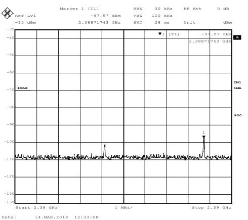
Figure 20 - Band-edge Measurement, Low Channel, Restricted Frequency, Radiated Measurement The plot shows an uncorrected measurement, used for relative measurements only.
