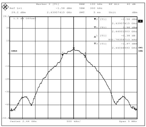
Figure 18 - 6dB Bandwidth, Mid Channel
