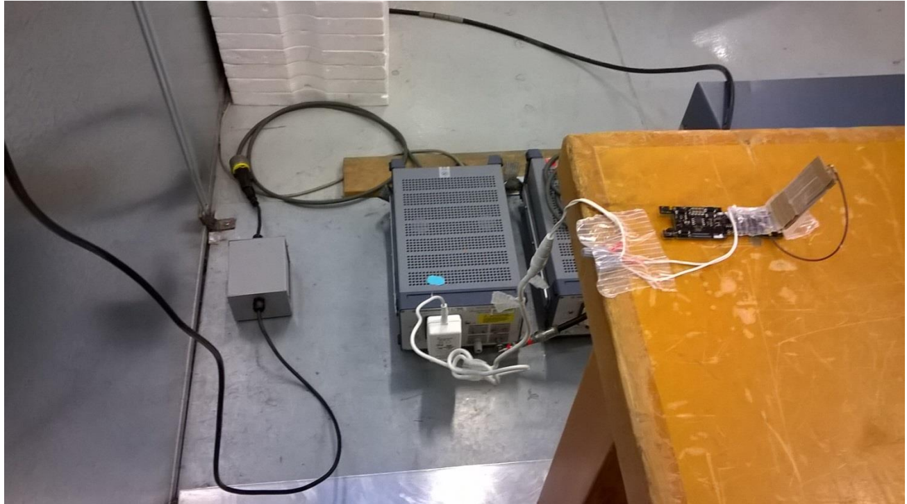
Figure 8 – Conducted Emissions Test Setup
