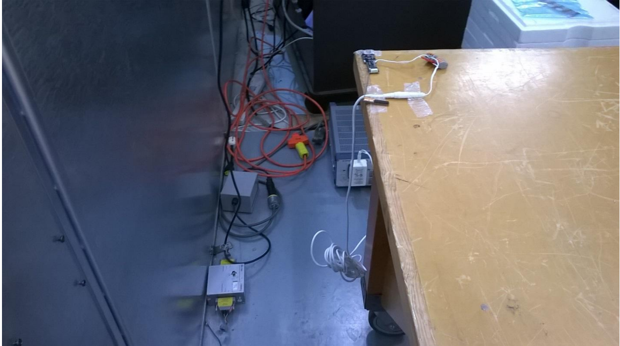
Figure 7 – AC Conducted emissions test setup d
