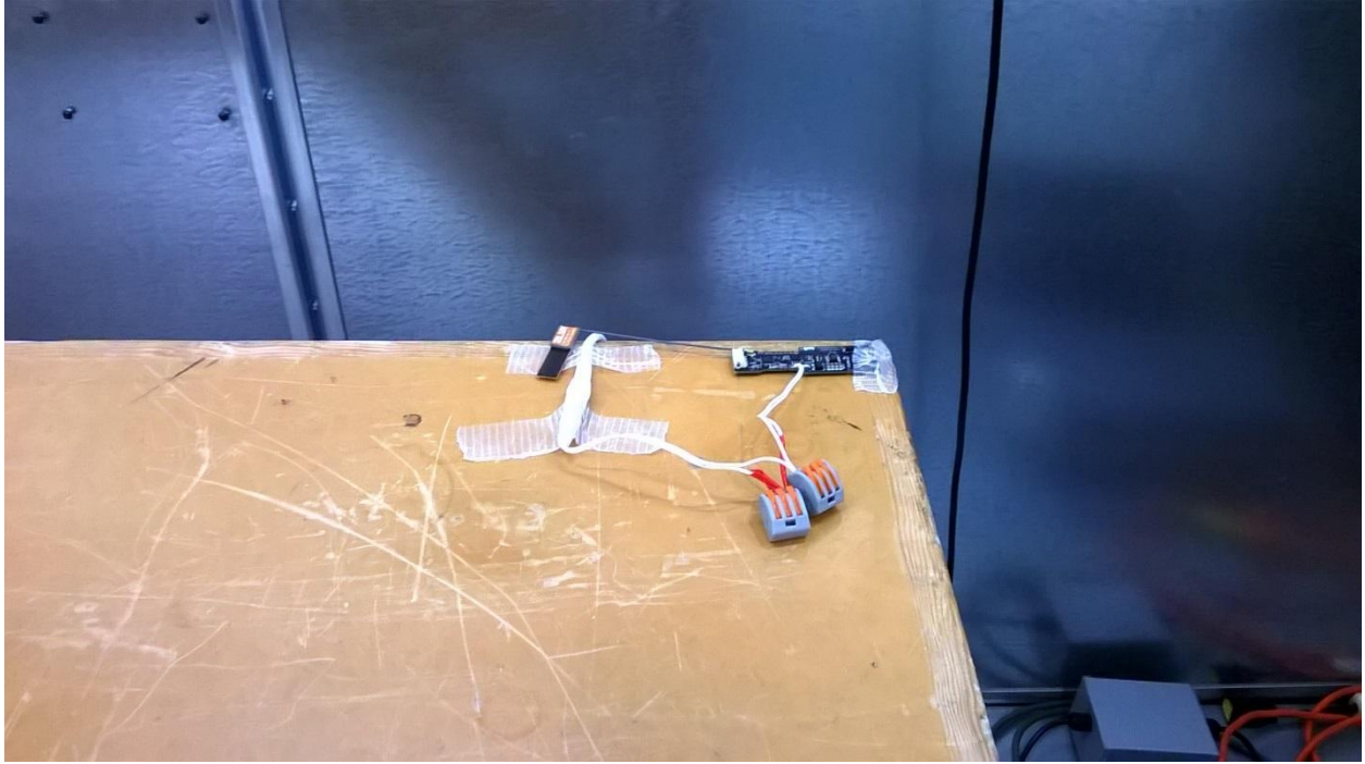
Figure 8 - AC Conducted Emissions Test Setup
