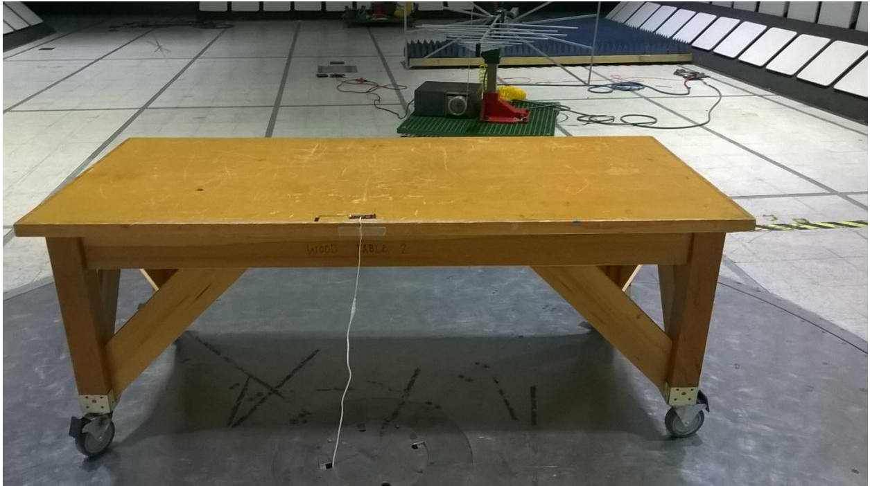
Figure 4 - Test Setup, 30M - 1GHz, Horizontal Orientation
