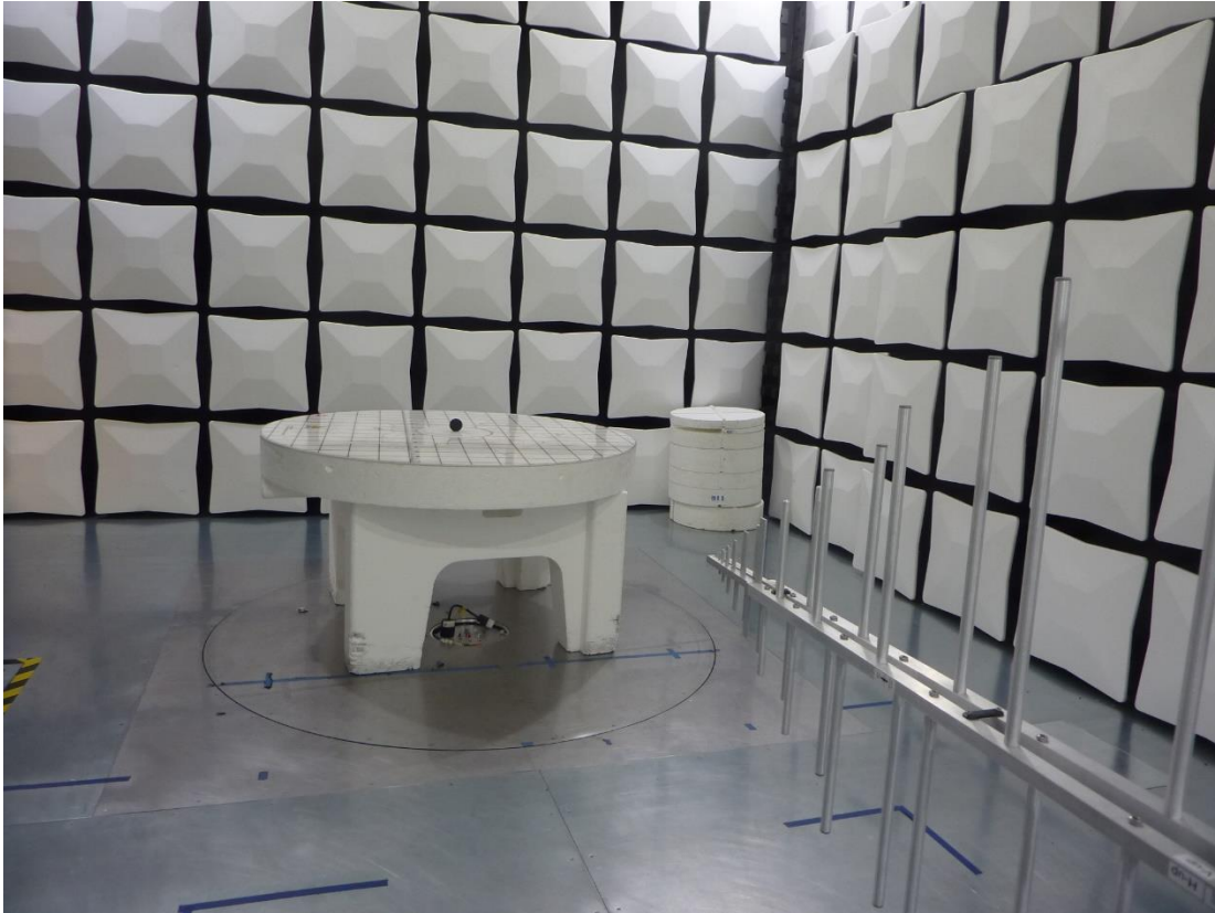
Figure 1: Test Setup for 30 MHz to 1 GHz (View 1)
