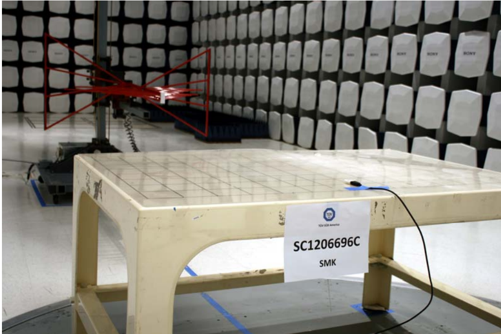
Radiated Emissions Test Setup (Below 1GHz)
