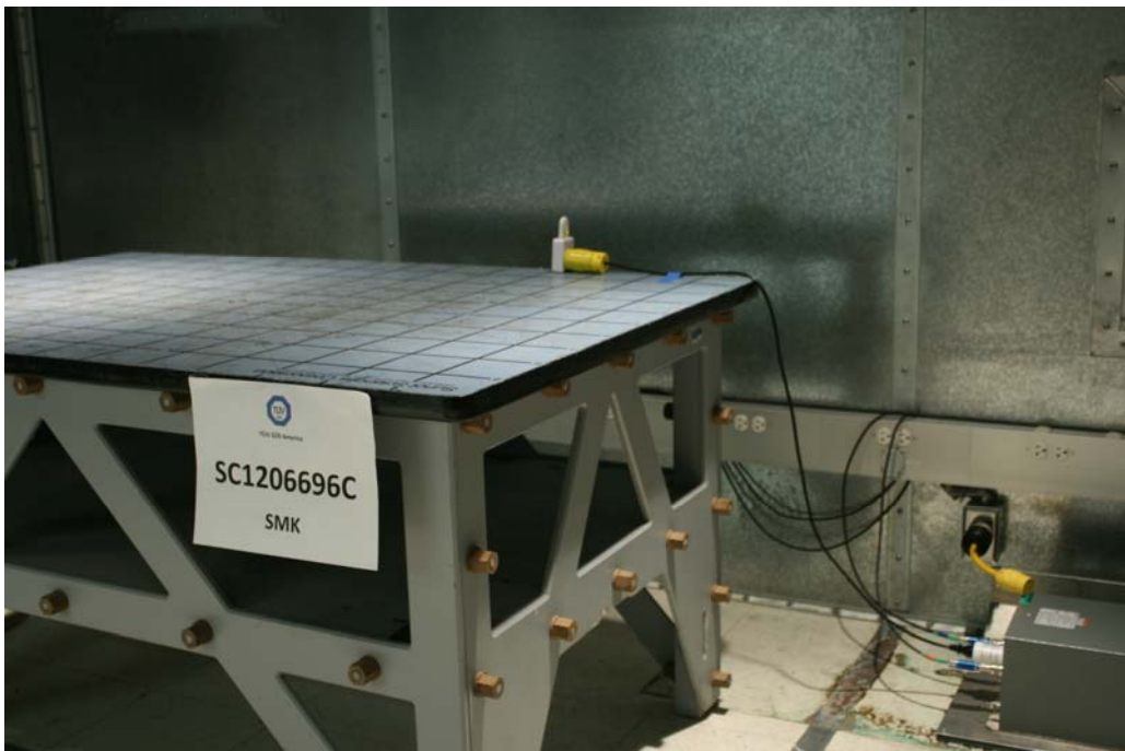
Conducted Emissions Test Setup
